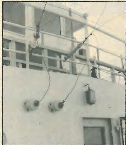
Fig. 7. Abbreviated version for a quick, cheap job on a 900-ton supply vessel failed repeatedly at sea. (Australian flag, photographed in Tasmania, 1976.)
