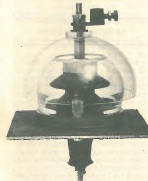
Fig. 13. Recently-developed British feedthrough assembly with dual-domed protective mantle. Moisture is expelled from domes by air blower. (By P. F. Barber, Scarborough.)
